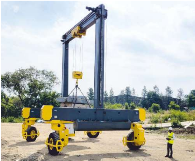
Pivoting motion using 2-wheel steering with 20t load
