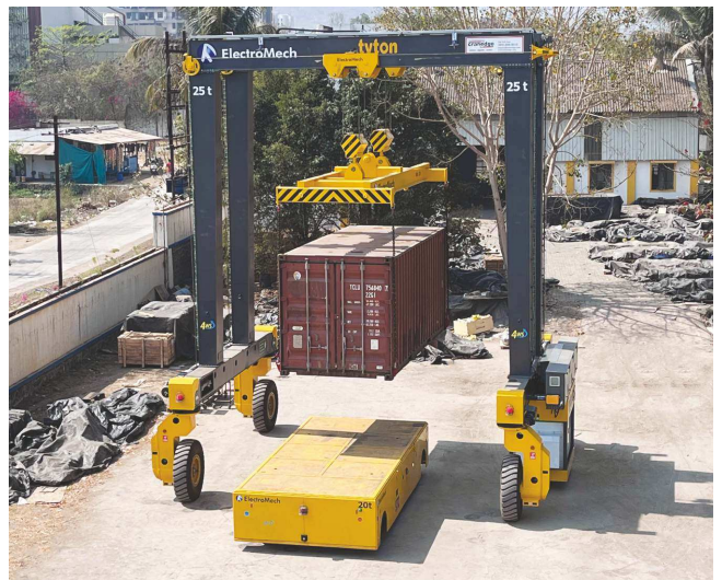
Handling of 20 feet shipping container
