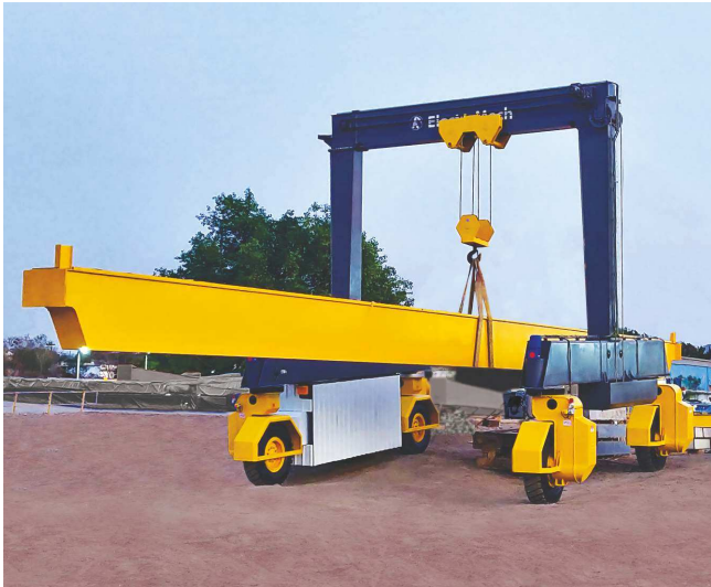
Long fabricated beam handling
